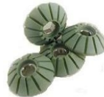
Fig. 4-3: Abrasive wheels fitted to a P556
