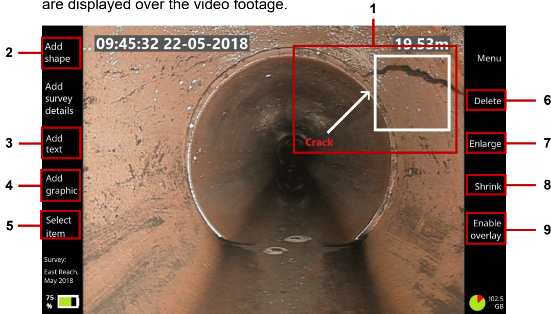
Fig. 6-30: Adding overlay items to a video recording. 1 Overlay text and shapes. Buttons: 2 Add shape. 3 Add text. 4 Add graphic. 5 Select item. 6 Delete item. 7 Enlarge item. 8 Shrink. 9 Enable overlay / Disable overlay.
