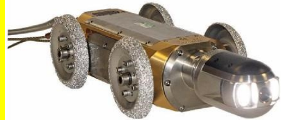
Fig. 4-3: Abrasive wheels fitted to a P556
