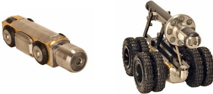
Fig. 3-9: P354 crawler with Forward View camera installed and P356 crawler with pan, tilt and zoom camera, large elevator and lighthouse installed.
