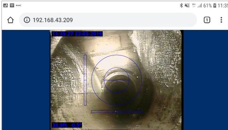
Fig. 6-22: Example of C550 controller display image streaming to a nearby device's display, here an Android phone's Chrome 72 browser
