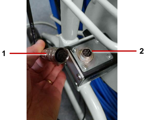
Fig. 4-23: Link cable (1) connects to the pushrod reel (2)
