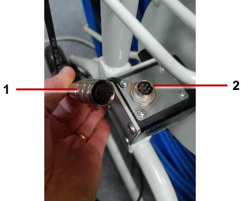
Fig. 4.23: Link cable (1) connects to the pushrod reel (2)
