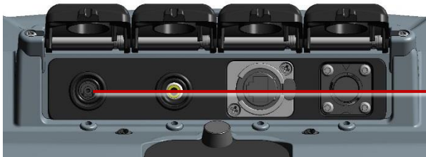
Fig. 4.31: Power socket (1) on main connection panel
