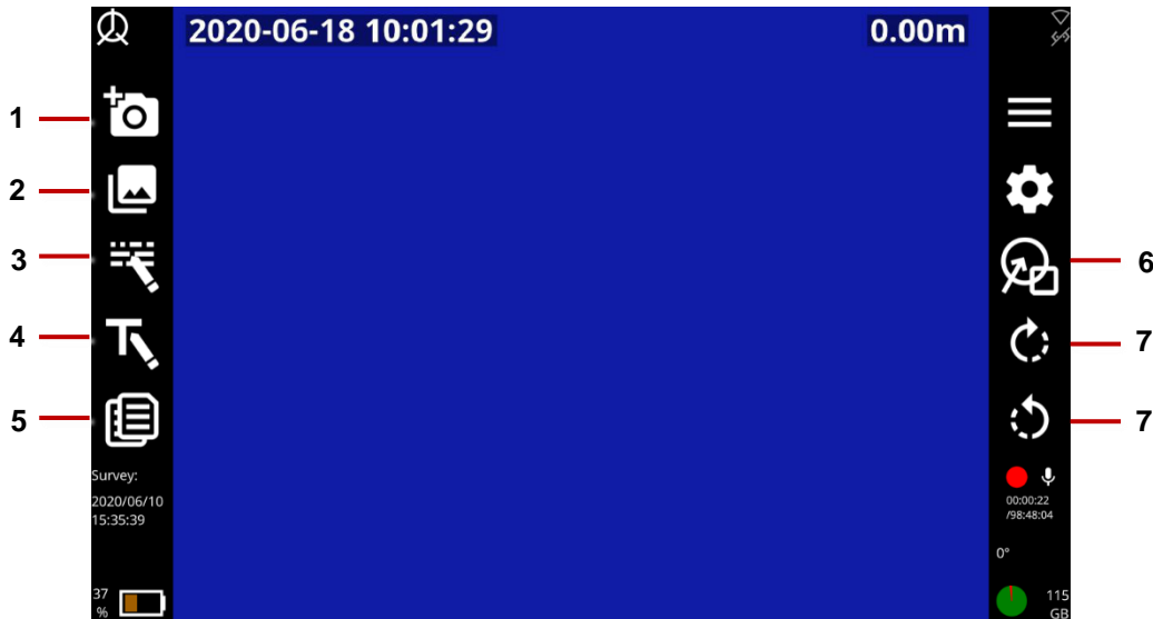
Fig. 7.2: Edit survey screen. 1 New observation button. 2 List observations button. 3 Edit survey header button. 4 Title page button. 5 Text pages button. 6 Overlay graphics button (for observations). 7 Roll camera buttons.
