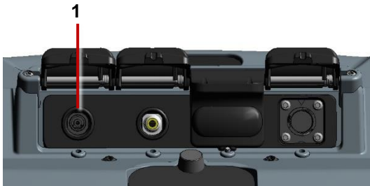
Fig. 4.10: Power socket (1) on main connection panel
