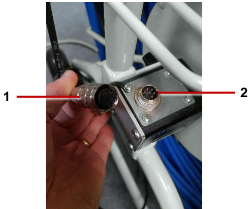
Fig. 4.2: Link cable (1) connects to the pushrod reel (2)
