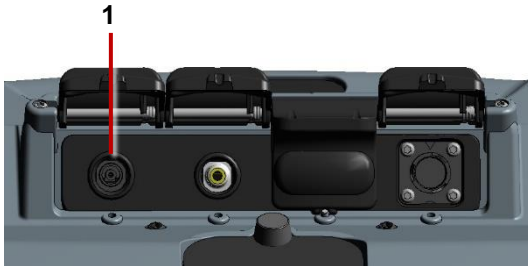
Fig. 4.10: Power socket (1) on main connection panel
