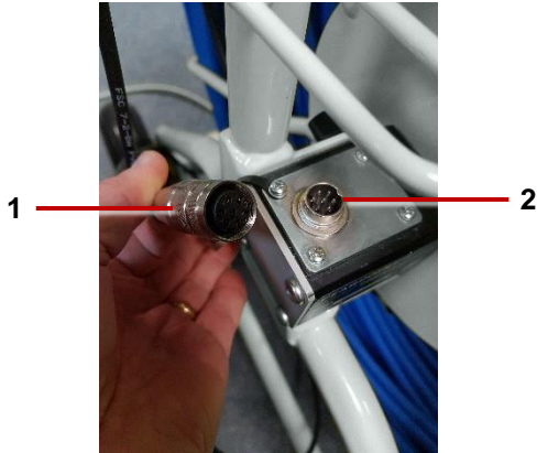
Fig. 4.2: Link cable (1) connects to the pushrod reel (2)
