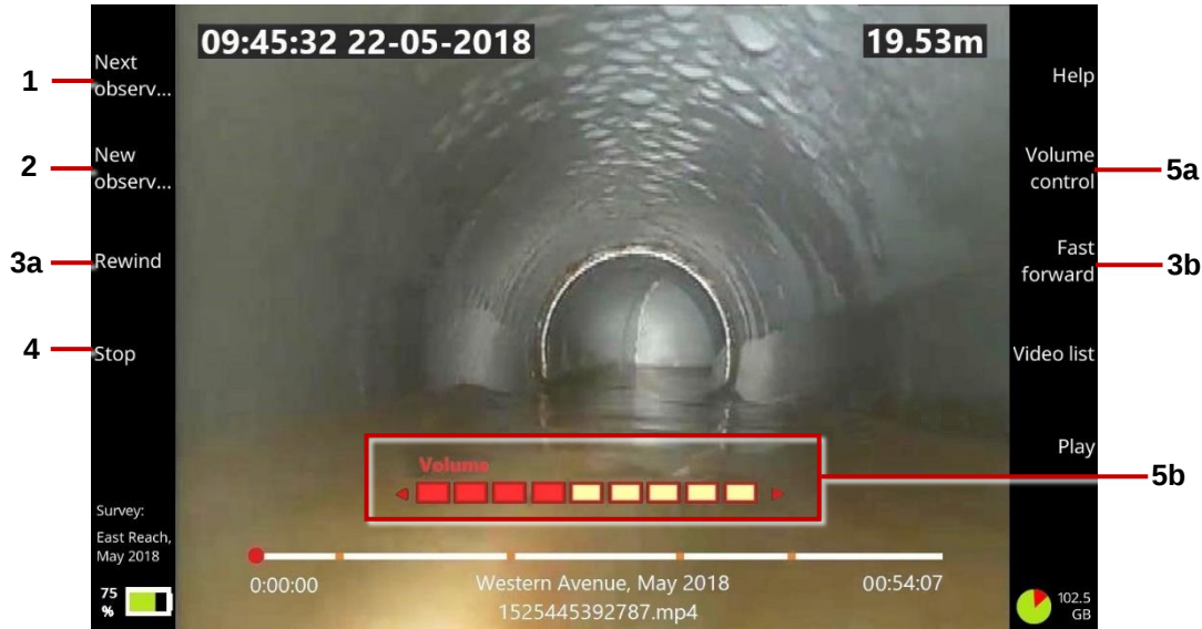
Fig. 6.7: Video playback screen. 1 Next observation button. 2 New observation button. 3a, 3b Rewind and Fast Forward buttons. 4 Stop button. 5a Volume Control button. 5b Volume level. Use the keyboard arrow keys to adjust the volume.
