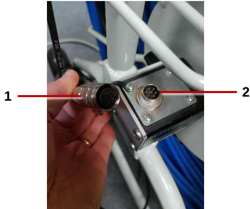
Fig. 4.2: Link cable (1) connects to the pushrod reel (2)
