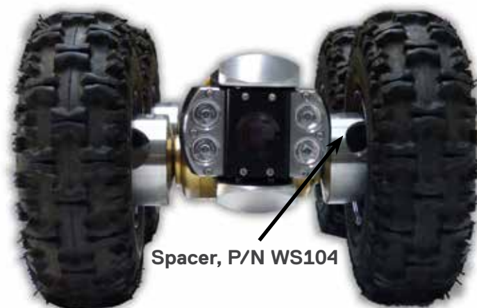
Steerable Pipe Ranger II Shown in the 18"+ Pipe Configuration
