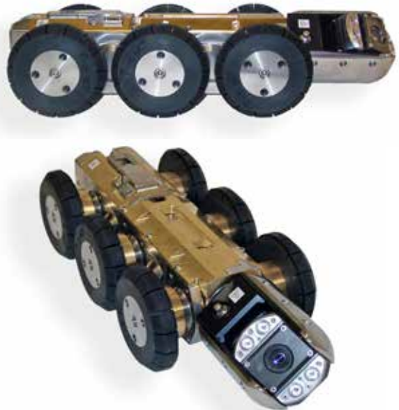
Compact Pipe Ranger (CPR) 10" Rubber Configuration
