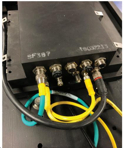
Apply dust caps to the receptacles that the strobe sync and DUC camera cable were plugged into.
