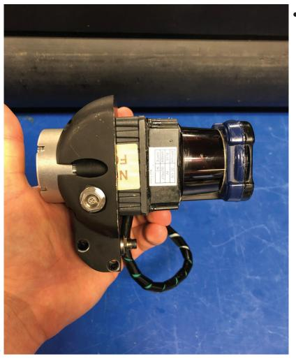
Install the LiDAR onto the back of the RVC with the four M3 screws that are bagged and tagged with the assembly.
