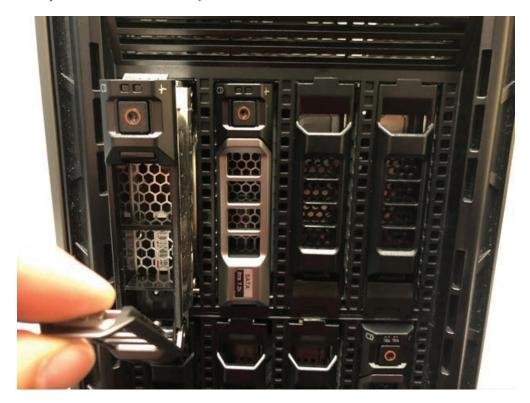
7. To remove the small blank hard drive covers, press the release tab on the top section of the holder.
