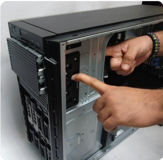
12. Once the bays are moved outwards, remove them from the front of the display by grabbing the sides and removing them one by one.
