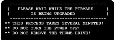
The system will copy in the new firmware release from the thumb drive and then reboot. The screen will change to:
