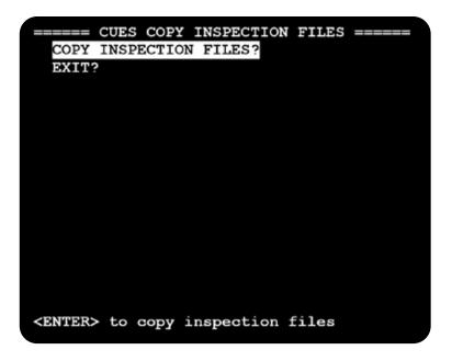
Label - COPY INSPECTION FILES? Type – Action Field Status line - <ENTER> to copy inspection files PRESS <ENTER> to copy the ID database file to a removable drive.
