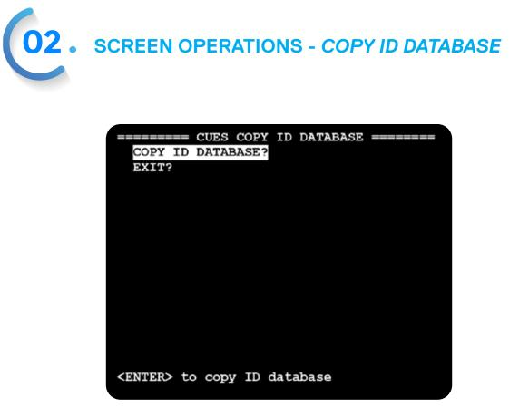
Label – COPY ID DATABASE? Type - Action Field Status Line – <ENTER> to copy ID database? Press <ENTER> to copy the ID database to a removable drive.
