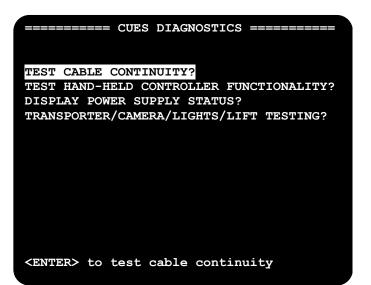
Label – TEST CABLE CONTINUITY? Type – Action Status Line – Test Cable Continuity? Press <ENTER> to move the operator to the Cable Continuity Screen.
