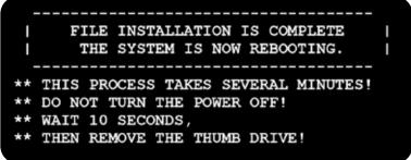
At the conclusion of the reboot, the system will now be running the new firmware release. This can be verified by viewing the release number on either the Copyright screen or the Equipment Configuration screen. The entire time for copying/rebooting/loading the new firmware can take a couple of minutes.
