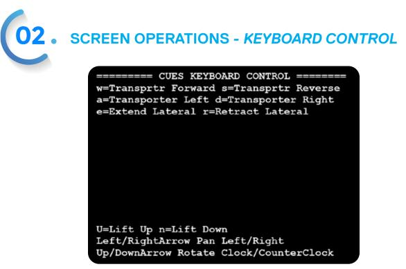
The Keyboard Control screen is available for controlling a limited (subset) of transporter, camera, lift and LAMPII functions, without using a game controller or Cues hand held controller. These keyboard controls could be used if the wireless gamepad stopped functioning (e.g. dead batteries) and there wasn't a wired gamepad available. In that situation, it would be desirable to retrieve the transporter which could be accomplished by first doing the following:
