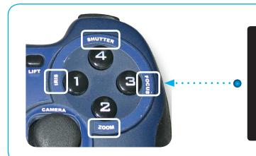
WHILE PRESSING THE IRIS BUTTON, SIMULTANEOUSLY PRESS THE PLUS / MINUS BUTTONS TO OPEN/CLOSE THE IRIS
