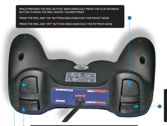
WHILE PRESSING THE LIGHTS BUTTON, SIMULTANEOUSLY PRESS THE PLUS OR MINUS BUTTON TO ILLUMINATE THE EXTERNAL LIGHTS BRIGHTER OR DIMMER
