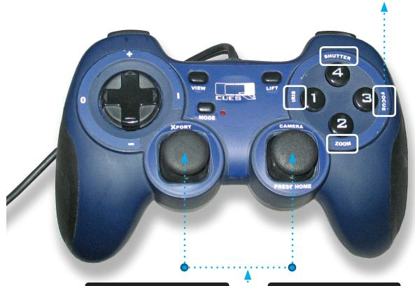
USE THE JOYSTICK TO MOVE THE TRANSPORTER. PRESS TO STOP THE TRANSPORTER.
