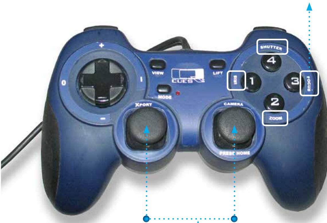
USE THE JOYSTICK TO MOVE THE TRANSPORTER. PRESS TO STOP THE TRANSPORTER.
