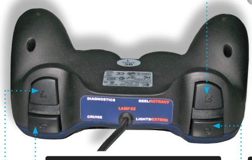
PRESS IN COMBINATION WITH THE DPAD 1 TO TURN CRUISE CONTROL ON PRESS IN COMBINATION WITH THE DPAD 0 TO TURN CRUISE CONTROL OFF PRESS IN COMBINATTION WITH THE DPAD + TO RAISE THE CRUISE CONTROL VOLTAGE PRESS IN COMBINATION WITH THE DPAD - TO LOWER THE CRUISE CONTROL VOLTAGE
