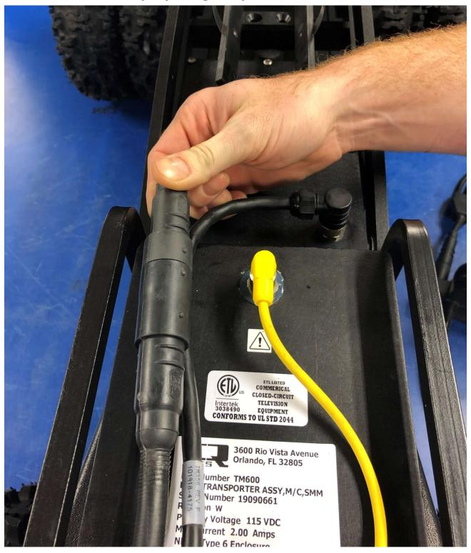
Install Dummy Plug, PN 160553, to the TM356 Cable.
