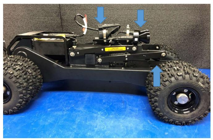
Remove auxiliary lights, mounting brackets, light cables, and Y-Eliminator.
