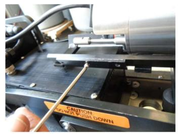
REMOVE REAR CLAMP AND INSTALL BRACKTES (HD102), ONE ON EACH SIDE, USING SCREWS (100448).
