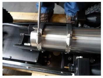
VERIFY THAT THE CAMERA SKIDS ARE STILL VERTICALLY ALIGNED WITH THE TRANSPORTER FRAME AND THAT THE CAMERA IS INSTALLED UPRIGHT. USE THE INDENTED AREA AT THE REAR OF THE CAMERA AS A GUIDE. TIGHTEN BOTH CAMERA CLAMPS.
