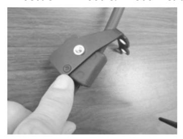
INSTALL HD308-2 CABLE SPLITTER. NOTE: BOSS ON SPLITTER MUST FIT INTO HOLE ON BRACKET.
