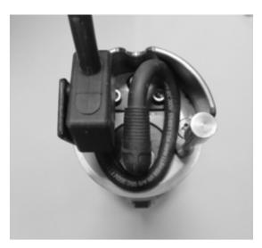
ROUTE AS SHOWN AND CONNECT HD308-2 CABLE TO THE CAMERA
