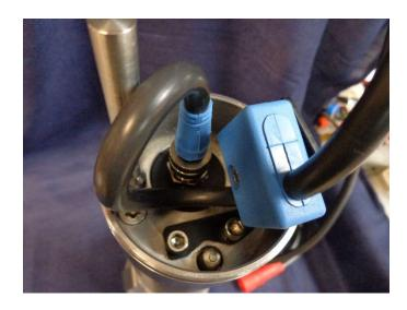
ROUTE AS SHOWN AND INSTALL BRACKET USING SCREWS, HW2353.
