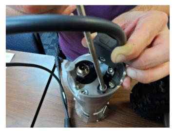
INSTALL BRACKET (HD047) AND SCREWS (HW2353), IF NECESSARY.
