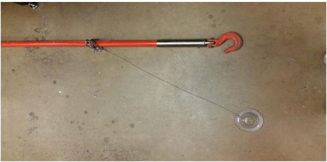
2. The flexible dome protector can be flexed to clear the front forks of the DUC, allowing the cover to sit directly on the DUC lens. The inside of the lens cover will fit directly around the black light shield ring.
