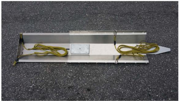
3. Position the Launcher Support Structure across the manhole with the cleats on the same side as the invert you are going to inspect. Position the launcher behind the Support Structure
