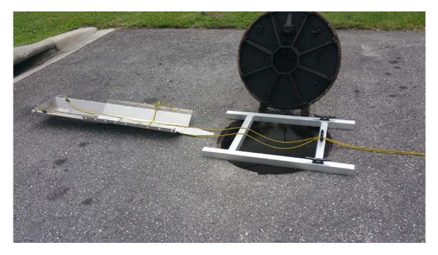
4. Pass the rear rope through the eyelet of the center cleat. Loop the rear rope around the cleat and pull tight as illustrated below. This step is a precautionary measure meant to attach the platform to the top side support structure in case the launcher is accidently dropped during positioning.
