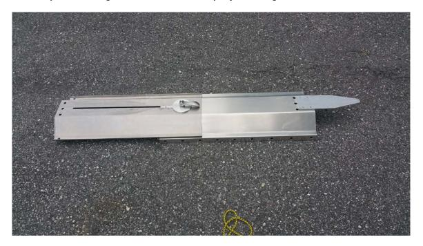
2. Attach one set of ropes across the rear of the Launcher and the other set across the front of the launcher. The further the offset is away from the opening of the manhole, the further back on the launcher platform you may need to attach the front rope.
