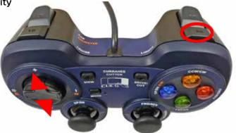
Hold down [LIGHTS] and press either [0] or [1] on the directional pad to raise or lower the spot light intensity in the cutting camera forks.
