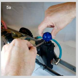
a. Attach the multi-conductor cable to the rear of the Cutter.
