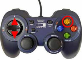
Hold down [FWD/REV] and press either [+] or [-] on the directional pad to increase or decrease the FWD/REV motor speed.
