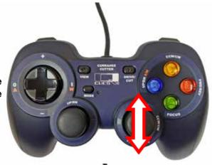
Move the right joystick left and right to rotate the cutting head counter-clockwise (CCW) and clockwise (CW).
