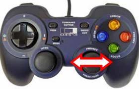
Move the left joystick forward and backward to adjust the cutting head upward (UP) and downward (DN).
