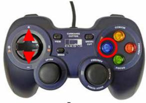
Hold down [CCW/CW] and press either [+] or [-] on the directional pad to increase or decrease the CCW/CW motor speed.
