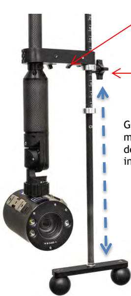
Pole Support Rod height can be adjusted with this thumb screw. Tighten thumbscrew when adjusting as required.
