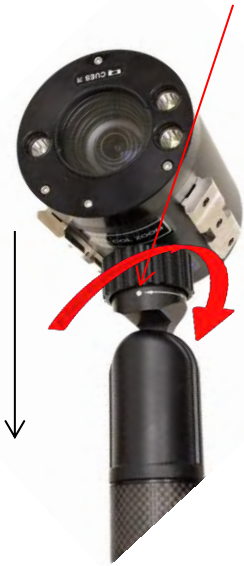
Camera UP orientation (for Left / Right panning)
