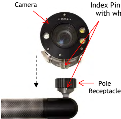
Insert Camera connector into Pole Receptacle
