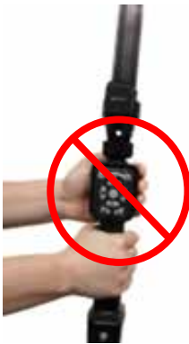
Improper hand position when holding pole facing upwards
