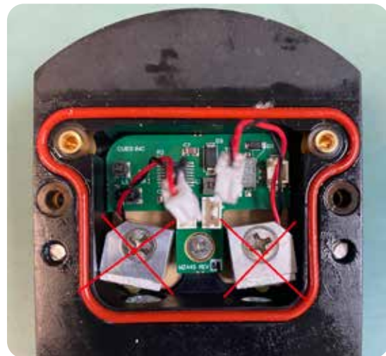
LED BLOCKS - INCORRECT ALIGNMENT
