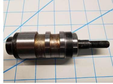
• CK353-1 AIR MOTOR CARTRIDGE, XL 3/8-24 SHFT
