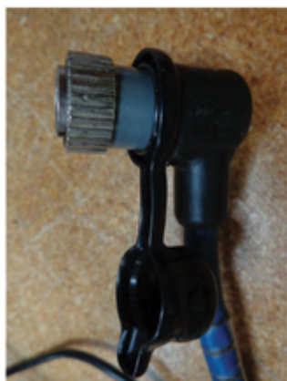
FIGURE 2.1 - EC2409 PROTECTIVE CAP (REF ONLY) PART OF CH900
