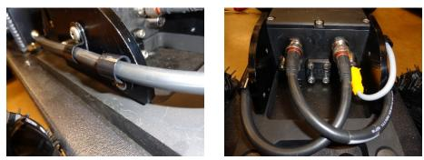
STEP 18- INSTALL TWO CABLE CLAMPS 121003 USING SCREWS 103031 ON THE LEFT WING OF THE TRANSMITTER FOR THE HD347 CABLE.
