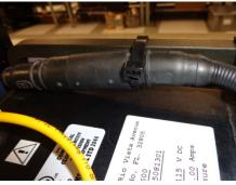
STEP 35- CONNECT THE 5 PIN DUMMY PLUG 160553 TO THE TRANSPORTER CABLING.
