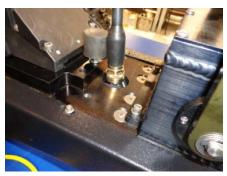
STEP 19- INSERT THE SONAR CABLE THROUGH THE FRONT HOLE IN THE CHASSIS.
