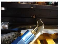
STEP 29- CONNECT THE SONAR CABLE TO THE SONAR HEAD. VERIFY THAT THE CONNECTOR GETS PLUGGED IN ALL THE WAY.
