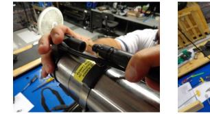
STEP 36- CONNECT THE DUAL LIGHT CABLE 160627 TO THE Y-ELIMINATOR WS123. NOTICE CABLE ROUTING.
