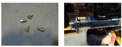
STEP 30- INSTALL THE SONAR GUARD AND TIGHTEN ALL FOUR MOUNTING SCREWS 101250 IN THE FRONT AND UNDER THE TRANSPORTER. *NOTE: USE THE FOUR FRONT HOLES OF THE TRANSPORTER.*
