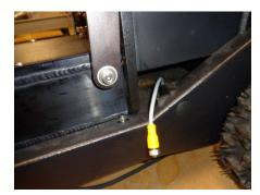
STEP 21- ROUTE THE CAMERA EXTENSION CABLE IN THE CHANNEL AND INSERT IT THROUGH THE REAR HOLE IN THE CHASSIS.
