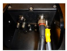
STEP 15- CONNECT THE CAMERA EXTENSION P/N EC2612 TO THE "CAM" CONNECTOR ON THE TRANSMITTER BOX.
