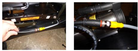
STEP 38- CONNECT THE CAMERA EXTENSION CABLE EC2612 TO THE Y-ELIMINATOR WS123.
