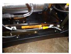
STEP 39- INSTALL TWO SMALL TIE WRAPS CS444 TO SECURE THE Y ELIMINATOR AND CAMERA EXTENSION CABLE TO THE STICY TIE WRAP MOUNTS.
