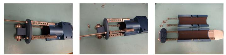
STEP 24- REMOVE THE TWO FRONT SCREWS AND SEPARATE THE TOP SONAR CLAMP FROM THE BOTTOM SONAR CLAMP WITH THE WHEELS.
