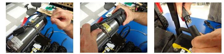
STEP 3- REMOVE THE THREE SET SCREWS IN THE BACK OF THE CAMERA AND REMOVE THE Y-ELIMINATOR AND UNPLUG Y-ELIMINATOR FROM THE 5 PIN CONNECTOR.
