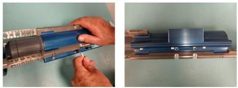
STEP 28- INSTALL ALL SIX SCREWS HOLDING THE TWO CLAMPS TOGETHER. THEN TIGHTEN THE TWO FRONT SCREWS.
