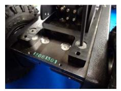
STEP 10- INSTALL THE TWO FRONT EXTERNAL SCREWS 101238.
