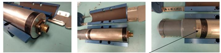
STEP 25- PLACE THE SONAR HEAD ON THE TOP SONAR CLAMP. *NOTE: PLACE THE SONAR WITH THE MARKING AWAY FROM THE CLAMP.*
