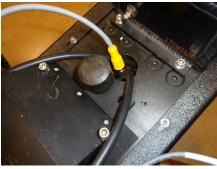
STEP 20- INSERT THE CAMERA EXTENSION CABLE THROUGH THE FRONT HOLE IN THE CHASSIS.
