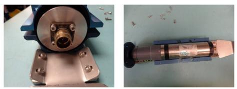
STEP 26- GRAB THE SONAR AND THE TOP CLAMP AND PLACE IT ON TOP OF THE BOTTOM CLAMP. **NOTE: IN THE RIGHT PICTURE, THE TOP CLAMP WAS REMOVED TO SHOW HOW THE SONAR SHOULD SEAT ON THE BOTTOM CLAMP.**
