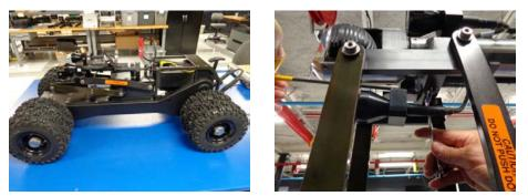
STEP 1- BRING THE LIFT UP AND REMOVE THE BOTTOM EXTERNAL LIGHTHEAD.
