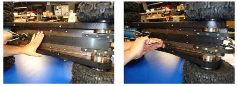
STEP 31- INSTALL THE CHANNEL PLATE SF726 USING SCREWS 103065.
