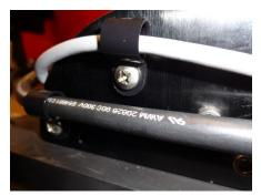
STEP 17- INSTALL TWO CABLE CLAMPS 121003 USING SCREWS 103031 ON THE RIGHT WING OF THE TRANSMITTER; ONE FOR THE SONAR CABLE AND ONE FOR THE CAMERA EXTENSION CABLE AS SHOWN.
