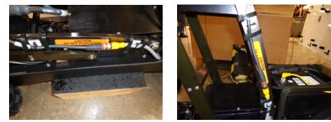
STEP 40- INSTALL FOUR LARGE TIE WRAPS 440304 TO SECURE THE Y ELIMINATOR AND CAMERA EXTENSION CABLE TO THE LIFT ARM.
