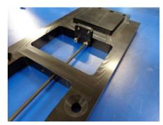
STEP 6- LOOSELY INSTALL THE SF288-1 PLATE TO THE SF720 PLATE USING SCREWS 101001.
