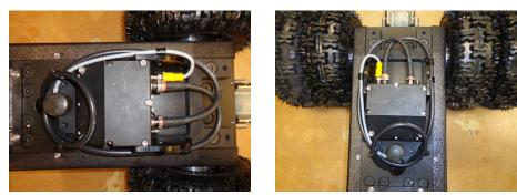
STEP 22- LOOP THE SF342 SONAR CABLE AROUND THE BUMPER AND PLACE TWO TIE WRAPS 440305 SECURING THEM TO THE CAMERA EXTENSION CABLE AND TO THE HD347 CABLE.
