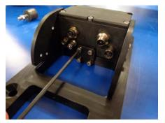
STEP 7- PLACE THE TRANSMITTER SF601 ON THE SF720 PLATE AND LOOSELY INSTALL THE TWO REAR SCREWS 102001 ON THE TRANSMITTER.
