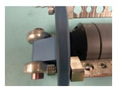
STEP 26- LOOSELY INSTALL THE TWO FRONT SCREWS BY HAND.
