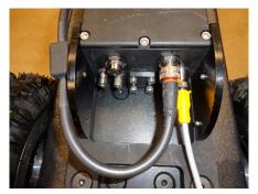
STEP 15- CONNECT THE CAMERA EXTENSION P/N EC2612 TO THE "CAM" CONNECTOR ON THE TRANSMITTER BOX.
