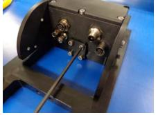
STEP 8- INSTALL AND TIGHTEN THE TWO FRONT SCREWS 104044 AND THEN TIGHTEN THE FOUR REAR SCREWS ON THE TRANSMITTER.
