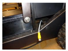
STEP 20- ROUTE THE CAMERA EXTENSION CABLE IN THE CHANNEL AND INSERT IT THROUGH THE REAR HOLE IN THE CHASSIS.
