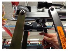
STEP 1- BRING THE LIFT UP AND REMOVE THE BOTTOM EXTERNAL LIGHTHEAD.
