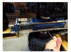
STEP 29- INSTALL THE SONAR GUARD AND TIGHTEN ALL FOUR MOUNTING SCREWS 101250 IN THE FRONT AND UNDER THE TRANSPORTER. **NOTE: USE THE FOUR FRONT HOLES OF THE TRANSPORTER.**
