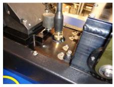
STEP 18- INSERT THE SONAR CABLE THROUGH THE FRONT HOLE IN THE CHASSIS.
