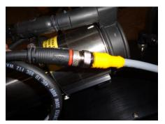
STEP 37- CONNECT THE CAMERA EXTENSION CABLE EC2612 TO THE Y-ELIMINATOR WS123.
