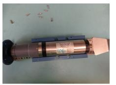
STEP 25- GRAB THE SONAR AND THE TOP CLAMP AND PLACE IT ON TOP OF THE BOTTOM CLAMP. **NOTE: IN THE RIGHT PICTURE, THE TOP CLAMP WAS REMOVED TO SHOW HOW THE SONAR SHOULD SEAT ON THE BOTTOM CLAMP.**
