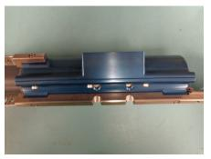
STEP 27- INSTALL ALL SIX SCREWS HOLDING THE TWO CLAMPS TOGETHER. THEN TIGHTEN THE TWO FRONT SCREWS.
