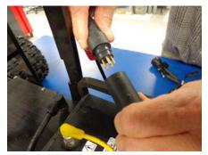
STEP 3- REMOVE THE THREE SET SCREWS IN THE BACK OF THE CAMERA AND REMOVE THE Y-ELIMINATOR AND UNPLUG Y-ELIMINATOR FROM THE 5 PIN CONNECTOR.
