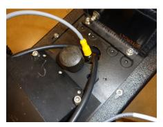
STEP 19- INSERT THE CAMERA EXTENSION CABLE THROUGH THE FRONT HOLE IN THE CHASSIS.
