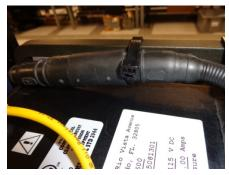
STEP 34- CONNECT THE 5 PIN DUMMY PLUG 160553 TO THE TRANSPORTER CABLING.
