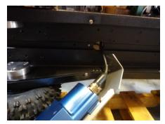
STEP 28- CONNECT THE SONAR CABLE TO THE SONAR HEAD. VERIFY THAT THE CONNECTOR GETS PLUGGED IN ALL THE WAY.
