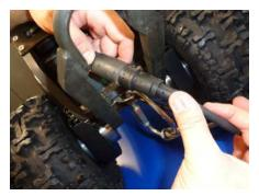
STEP 32- PLUG THE 12 PIN END OF THE HD342-2 CABLE TO THE TRANSPORTER CABLING.
