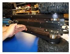
STEP 30- INSTALL THE CHANNEL PLATE SF726 USING SCREWS 103065.
