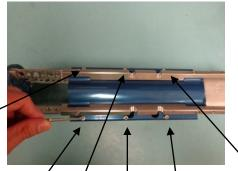
STEP 22- REMOVE THE SIX SCREWS HOLDING THE TWO BLUE SONAR CLAMPS TOGETHER ON THE SONAR GUARD SF386.
