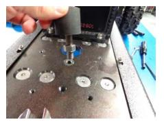
STEP 4- LOOSEN THE BUMPER NUT AND REMOVE THE BUMPER.
