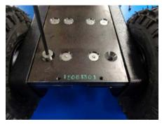
STEP 5- REMOVE THE TWO FRONT EXTERNAL SCREWS.
