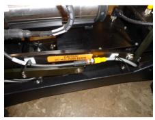
STEP 38- INSTALL TWO SMALL TIE WRAPS CS444 TO SECURE THE Y ELIMINATOR AND CAMERA EXTENSION CABLE TO THE STICY TIE WRAP MOUNTS.
