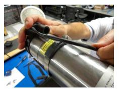
STEP 33- PLUG THE Y-ELIMINATOR WS123 TO THE CAMERA. AND TIGHTEN THE THREE SET SCREWS.
