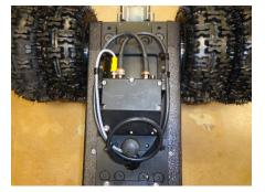
STEP 21- LOOP THE SF342 SONAR CABLE AROUND THE BUMPER AND PLACE TWO TIE WRAPS 440305 SECURING THEM TO THE CAMERA EXTENSION CABLE AND TO THE HD342-2 CABLE.
