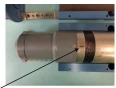
STEP 24- PLACE THE SONAR HEAD ON THE TOP SONAR CLAMP. **NOTE: PLACE THE SONAR WITH THE MARKING AWAY FROM THE CLAMP.**
