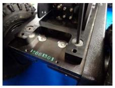
STEP 10- INSTALL THE TWO FRONT EXTERNAL SCREWS 101238.
