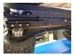
STEP 12- INSERT THE HD12 END OF THE HD342-2 CABLE THROUGH THE TOP OF THE FRONT HOLE ON THE SMM AND ROUTE TOWARDS THE BACK OF THE TRANSPORTER IN THE CHANNEL.
