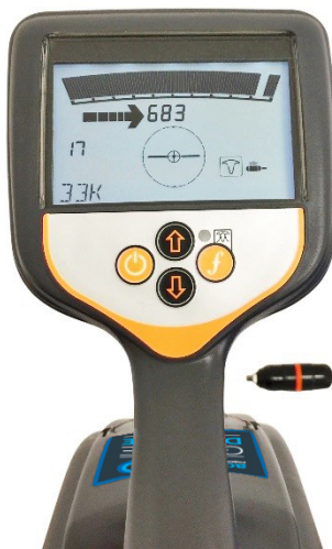
Figure 4.9: Locator in Guidance mode with 33 kHz standard sonde
