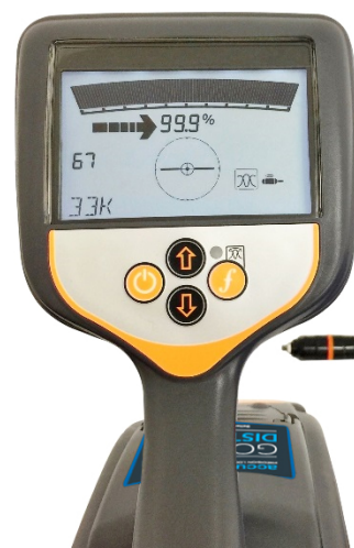
Figure 4.8: Locator in Peak+ Guide mode with 33 kHz standard sonde
