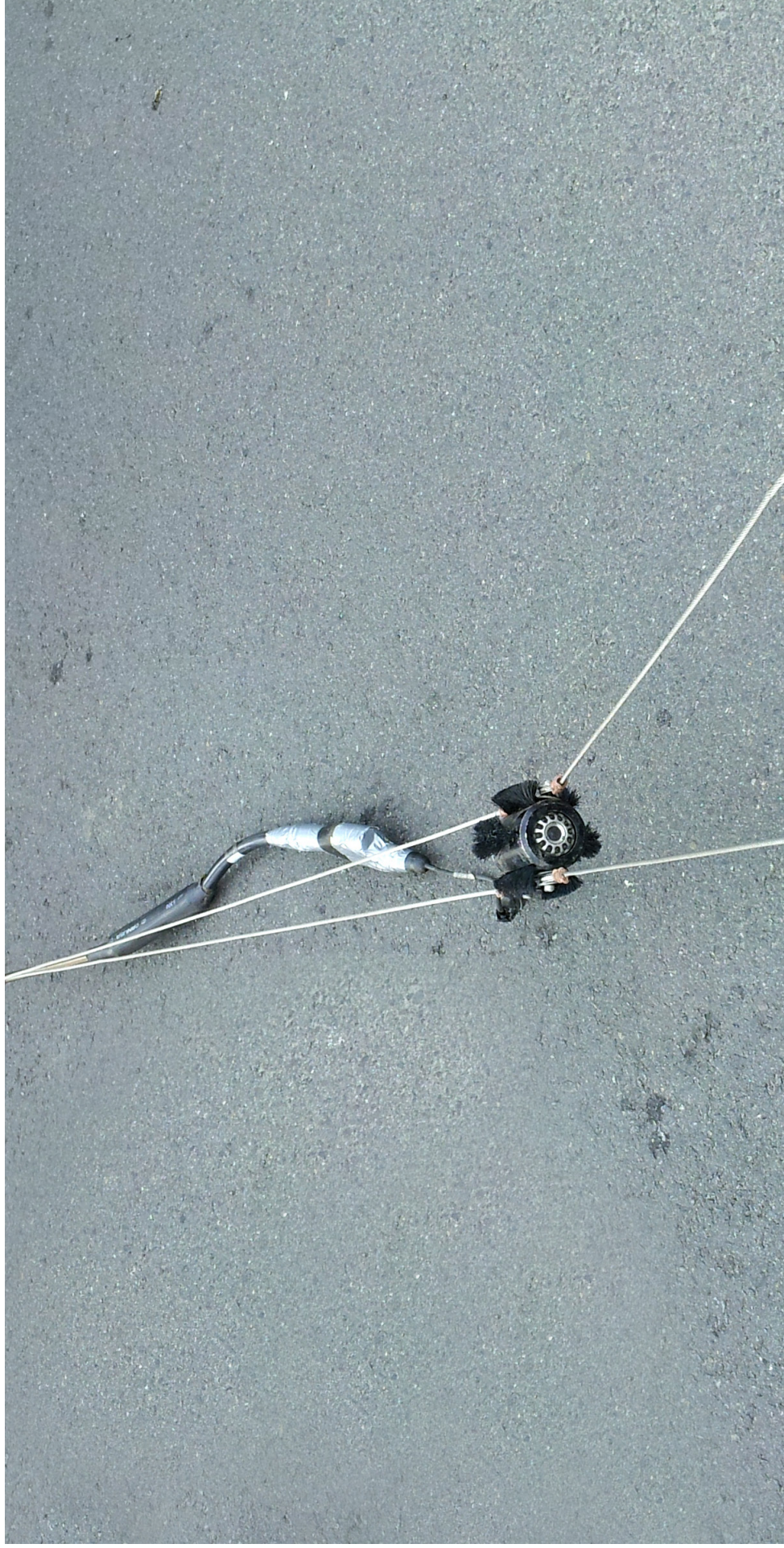
Figure 1: ProScout Camera with Centralizing Brush Assembly
