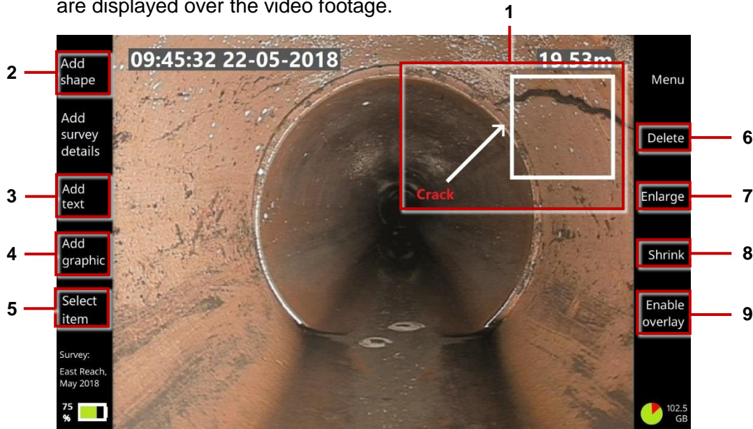
Fig. 6.24: Adding overlay items to a video recording. 1 Overlay text and shapes. Buttons: 2 Add shape. 3 Add text. 4 Add graphic. 5 Select item. 6 Delete item. 7 Enlarge item. 8 Shrink. 9 Enable overlay / Disable overlay.
