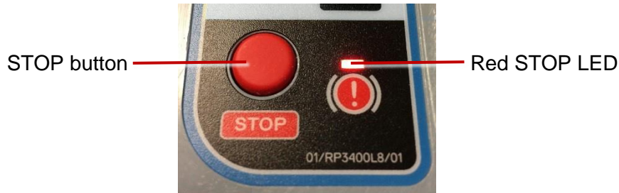
Fig. 6.11 STOP button and red STOP LED
