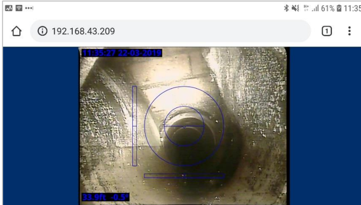
Fig. 6.22: Example of P550 controller display image streaming to a nearby device's display, here an Android phone's Chrome 72 browser
