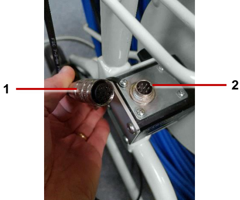
Fig. 4.23: Link cable (1) connects to the pushrod reel (2)
