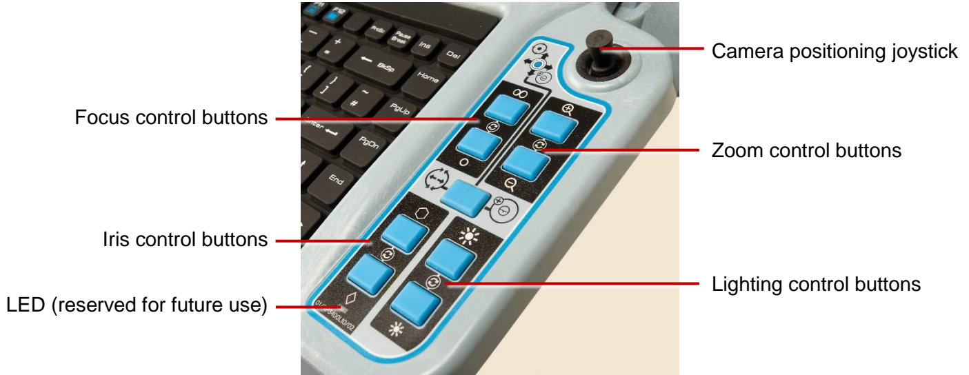
Fig. 6.16 Right hand joystick and camera & lighting control buttons
