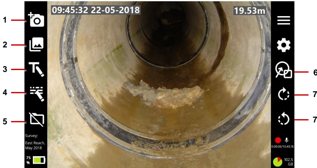
Fig. 7.2: Edit survey screen. 1 New observation button. 2 List observations button. 3 Title page button. 4 Edit survey header button. 5 Close survey button. 6 Overlay graphics button (for observations). 7 Roll camera buttons.
