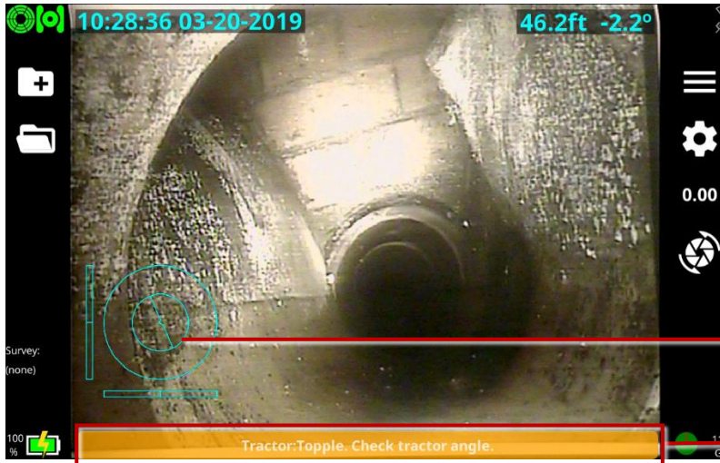
Fig. 6.14 Topple warning shows at the bottom of the screen. Note that the MIMIC also shows a high tilt angle.
