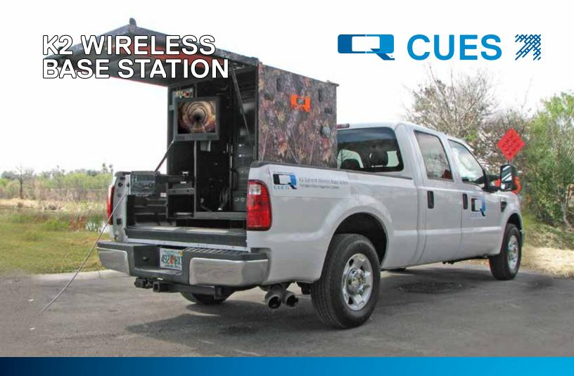
THE CUES K2 BASE STATION IS MOUNTED IN A COMPACT, RUGGED, WEATHER-PROOF ENCLOSURE AND CAN FIT INTO AN ATV, VAN, OR PICK-UP TRUCK TO ACCESS EASEMENTS AND HARD-TO-REACH AREAS.
