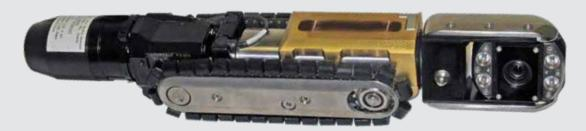
Ultra Shorty III features a reduced camera/tractor length with the CUES OZIII-S or OZ4-HD cameras to facilitate line entry through inverts with limited space and traverses 22, 45, and 90 degree sweeps in smaller diameter lines. The transporter includes weighted adapter blocks to optically center the camera and a built-in connector and protective housing for direct insertion of the optional OZIII-S or OZ4-HD cameras; no camera interface cables are required.
