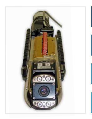
Inspect 6" (152 mm) relined to 24" (610 mm) lines with major offsets and protruding laterals.
