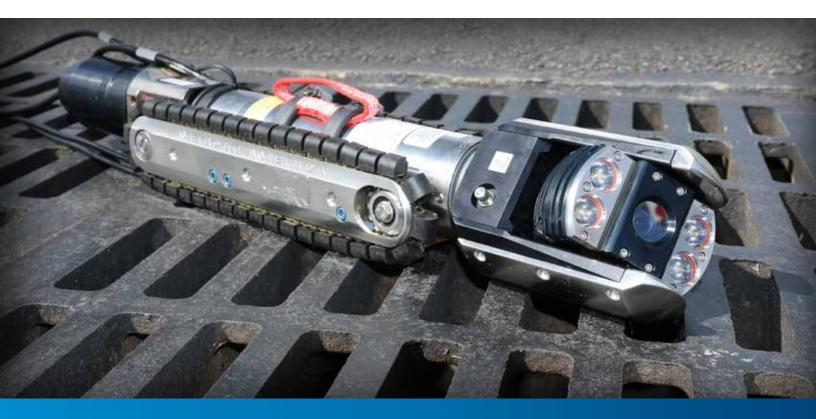
The CUES Ultra Shorty 21 is a trackedtransporter designed to inspect 6"- 36" (152 mm - 914 mm) lines with major offsets and protruding laterals. Adapter blocks are available to optically center the camera in 30"- 36" (762 mm - 914 mm) lines. The transporter, when combined with the OZII pan, tilt, optical zoom camera, offers a compact assembly at only 28" (711 mm).
