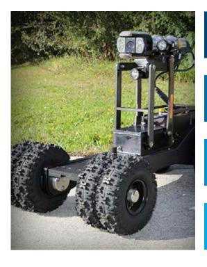
SMM is a self-propelled power forward, power reverse, and freewheel multiconductor transporter.
