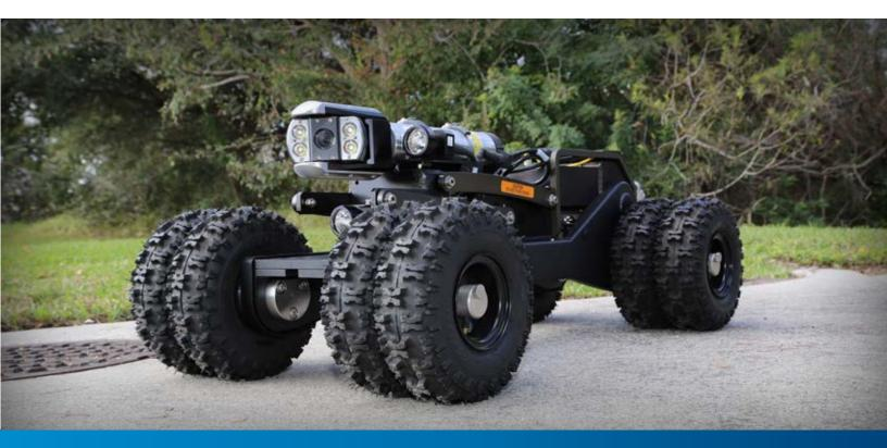
The Steerable Mudmaster is a camera transporter specifically designed with the necessary weight, power, high clearance, and all-wheel drive for pipelines ranging from 24"- 200" (610 mm - 5080 mm).
