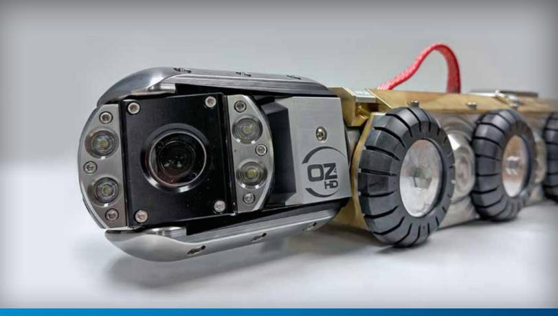
The OZ4-HD is a 1080p high-definition pan & tilt mainline camera. OZ4-HD provides up to 160:1 optical digital zoom, automatic focus, as well as remote focus and iris control, to assure the best quality video within varying pipe conditions.
