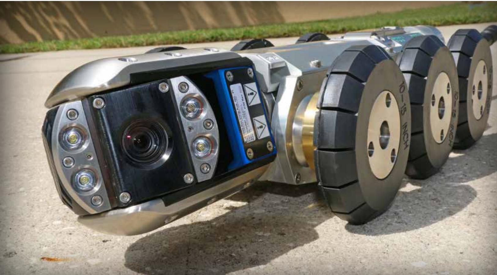
The OZIII-S camera provides up to 120:1 optical/digital zoom, automatic focus, as well as remote focus and iris control, to assure the best quality video within varying pipe conditions.
