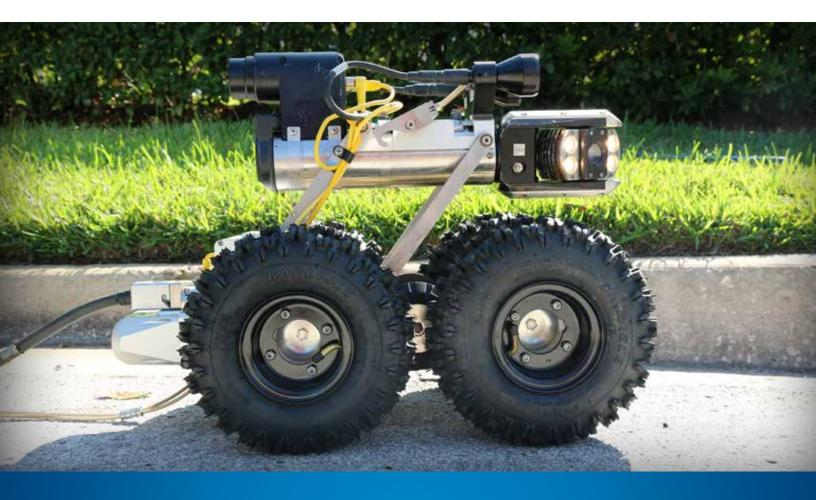
The OZII optical zoom pan-and-tilt camera offers unparalleled imaging technology and built-in lighting for 6"- 72" (152 -1829 mm) pipe to produce clarity of picture with enhanced detail.
