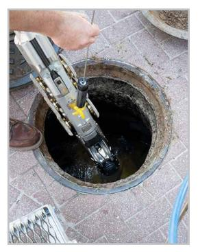
Built-in multi-frequency sonde transmitter; 512 Hz or 8 kHz.
