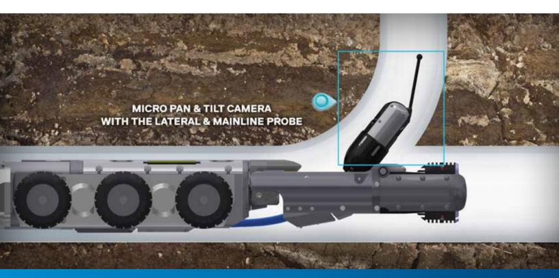
The CUES Micro Pan & Tilt Camera is designed to navigate through multiple wyes and 45 and 90 degree bends / sweeps with the integrated directional rod. All pan and tilt functionality is integrated into the systems' controller. The Micro Pan & Tilt Camera includes a detachable steering wand, self-leveling camera head, built-in lens wiper, 360 degrees pan and tilt, (2) banks of LED's with variable light intensity, and a built-in sonde with switchable frequencies.
