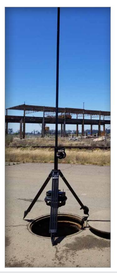
Perform manhole & mainline inspections and gauge the manhole depth without the need for a camera transporter!
