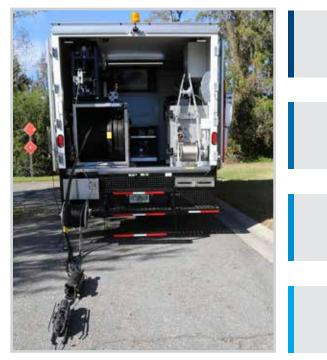
Low void packers are available for 8"- 20" (203 mm - 1067 mm) diameter pipe sizes. \*Larger sizes are available upon request.
