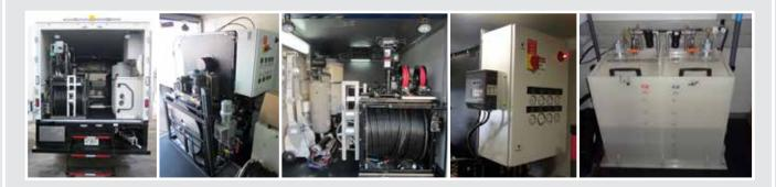
Other design features include the ability to air pre-test, grout seal, and re-test without the need for repositioning. Its low profile design insures a minimum grout ring residue remaining at the joint with maximum dispensing efficiency of the grout material.
