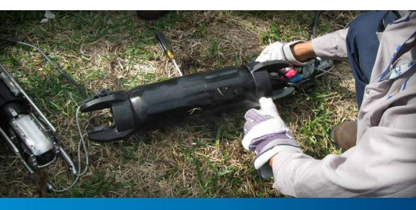
CUES Low Void Packers are low-volume, chemical injection, multi-grout packers. low volume packers work with acrylamides and other common chemical grouting materials.
