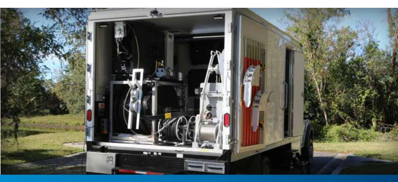
CUES offers a full line of CONTRACTOR-GRADE portable and truck-mounted chemical grout rehabilitation systems. Grout packers are available for mainline and lateral sealing. Truck-mounted grout rehabilitation systems are available for mainline joint sealing/lateral sealing and can be equipped with the latest CCTV equipment for television inspection. The system offers plenty of room for packers and grout materials.
