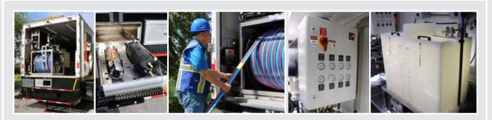
Applications include pipe stabilization and support, joint testing and sealing of mainline and lateral joints, manholes, junction boxes, large diameter pipes, or any other low pressure waterproofing application. All systems can be configured to run Acrylamide and Acrylate grouts. Dry freight box (for export),trailer-mounted systems, and retrofits are also available. Combo trucks are available for TV, Cutter, & Easy Grout.
