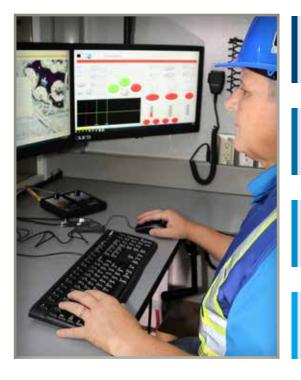
Modern look and feel; displays packer pressure, sleeve vacuum/pressure, pump speed, daily and per joint totalizers.
