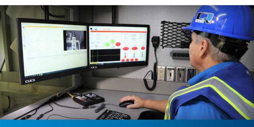
**NO MORE mechanical, analog, dials, switches, or buttons!** The CUES Easy Grout system is a computerized grout control system is designed to consolidate all the valves, electrical controls, etc., into an instrumentation cabinet that can be mounted in any location.
