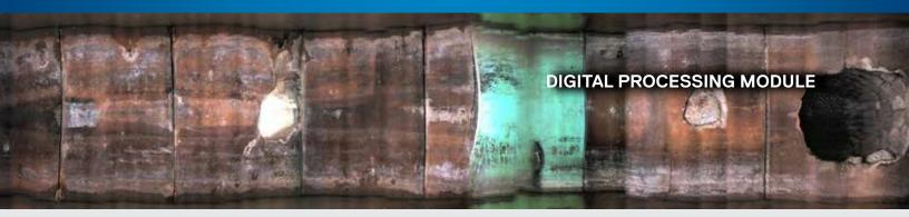
Video is stitched via the CUES GraniteNet software digital processing module. Flat images are available immediately following the inspection while LIVE video is available during/throughout the inspection. Virtual pan, tilt, and zoom plus a flat unfolded view of the entire surveyed pipe, enables rapid condition assessment review, significantly faster than traditional video inspection review. An expanded flat view is provided for additional detail with measuring capabilities.
