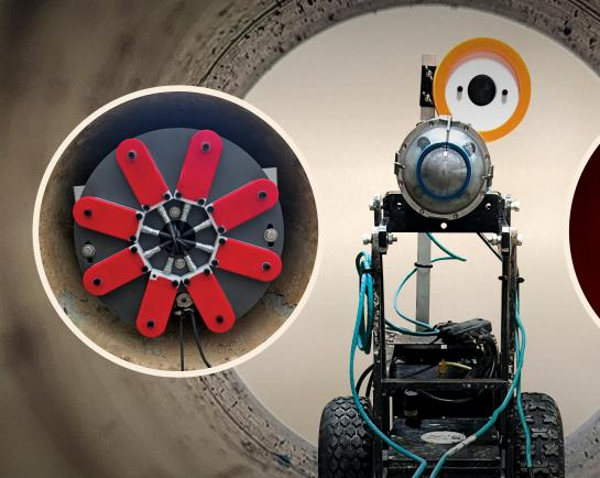
Electromagnetic testing delivers the most detailed condition data for large diameter concrete pressure pipelines in both early and advanced states of distress.
